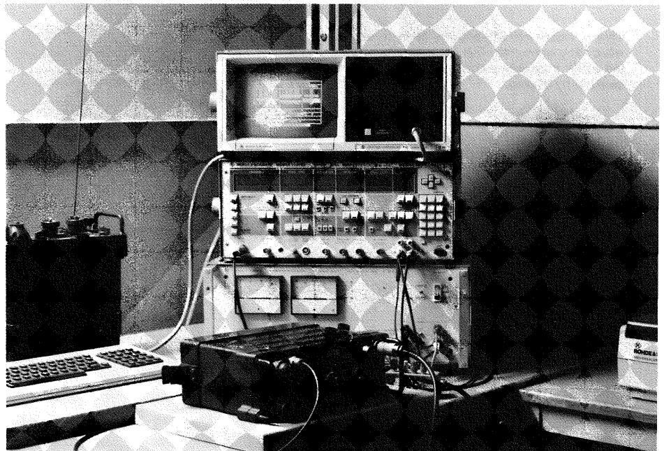
In the shielded cabin: a PRC-77 being tested by SMFP 2 and PUC. ▼
