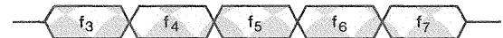
FIG 1 Simplest form of selective call, consisting of sequence of five equally long tones.
