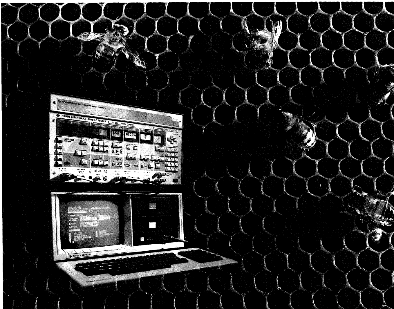
FIG 1 Automatic test assembly for mobile phones of cellular-radio networks AMPS, TACS and NMT, consisting of Radiocode Test Set SCUD and Mobile Tester SMFP 2 with Duplex Deviation Meter SMFP B41.
