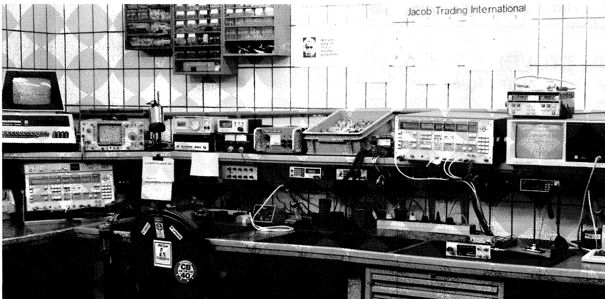
◀ SMFS 2 (with analog display), SCUD and NAP form the nucleus of the personal-radio test assembly for 934 MHz.
